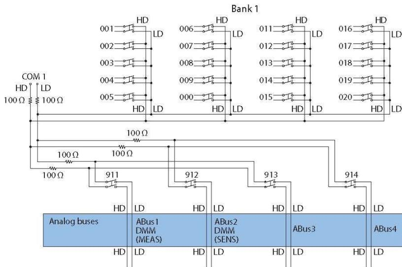
Figure 5. 34923A 40-channel reed multiplexer (bank 1 shown)
