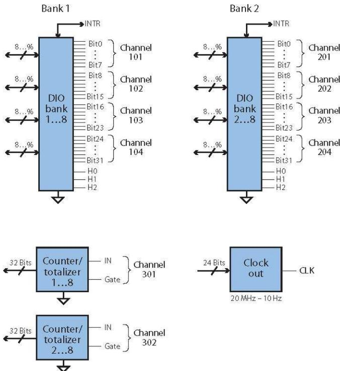
Figure 13. 34950A 64-channel digital I/O
