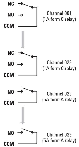
Figure 9. 34937A 32-channel Form A/ Form C switch
