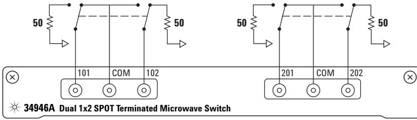
Figure 11. 34946A dual 1x2 SPDT terminated microwave switch
