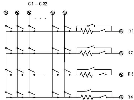
Figure 8. 34934A quad 4x32 matrix (1 of 4 matrices shown)
