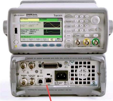
LAN (LXI Class C), USB and GPIB connectivity for quick and easy connectivity to a PC or network.
